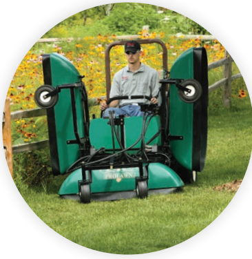
Side curtains fold up for tight spaces.
